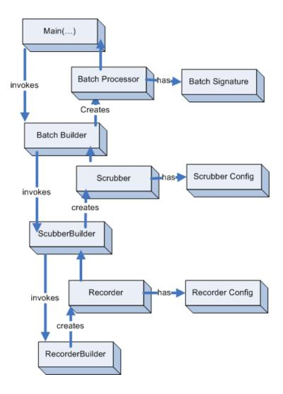
The configuration XML can be used to assemble a runtime collection of scrubber objects. In this diagram, each builder uses and consumes the product of the builder immediately below it.
