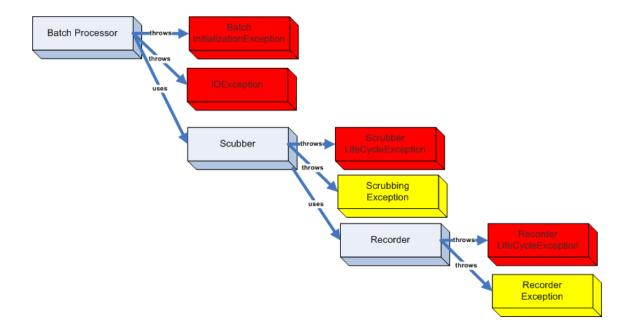
The **BatchProcessor** continues if a single file fails, but will abort if there is an error during initialization of the batch, scrubber, and recorder. The diagram above depicts the catched exceptions as *warnings* in  $\frac{\text{YELLOW}}{\text{Atal}}$  and the f atal exceptions in  $\frac{\text{RED}}{\text{RED}}$ .
